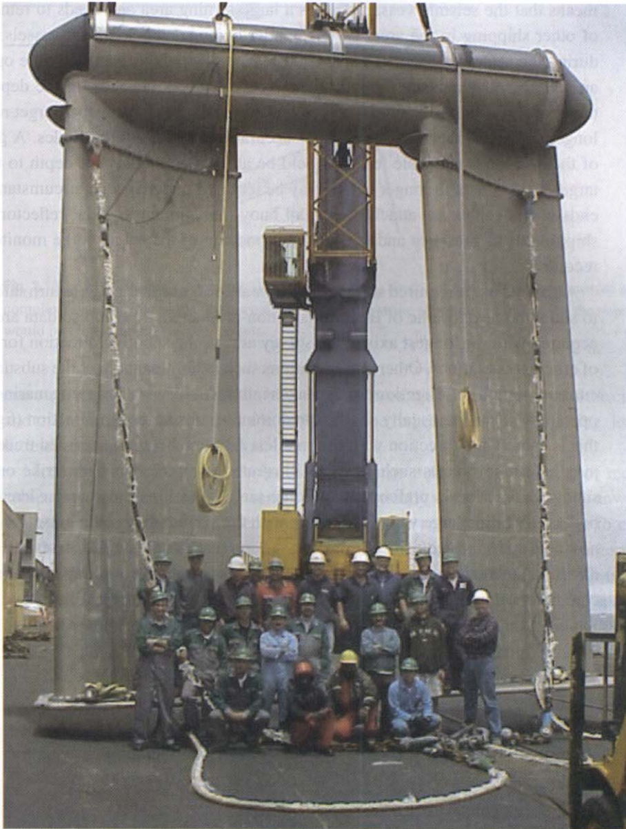
Fig. 2.8 A paravane used to control the position of the head of the receiver cable.
