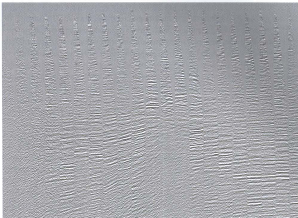
Fig. 2.34 Examination of CMP gathers during an iteration of pre-stack depth migration. Pre-stack depth migration is required in areas of complex lateral velocity variation. In such areas the standard normal moveout equation is insufficient to align events owing to the different paths that the waves take through the subsurface. In order to apply pre-stack depth migration one needs to supply the correct velocity–depth model. This is generally not known and so is built in an iterative fashion during the pre-stack migration. The correct velocity model is the one where the migrated gathers are flat across all offsets. Here we see gathers during a pre-stack migration iteration. Some of the events are flat, indicating that the correct model has been determined. Others are still dipping and the velocity model needs updating to flatten them also.
