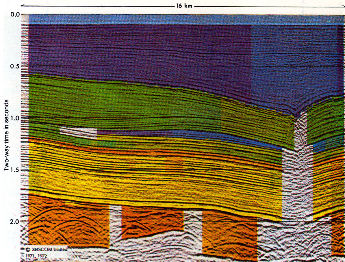
Figure 4/36 Colour coded interval velocities superimposed on a conventional North Sea section. Note the velocity gradient reversal at approximately 1.15 s in the centre of the section. Colour code as follows: computer interval velocity in ft/s: pale blue—5000; dark blue—5000–8500; dark green—8500–10500; pale green—10500–12000; yellow—12000–13000; orange—13000–15000. (Courtesy: Seiscom).
