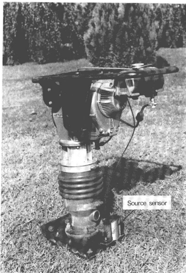
Figure 3/15 Mini-Sosie seismic source. A signature recording sensor is mounted on the top side of the vibrator base-plate. (Courtesy: Société Nationale Elf Aquitaine (Production): SNEA (P).)
