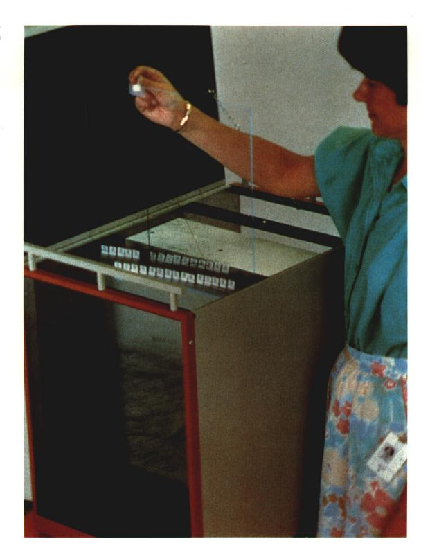
**Seiscrop section**. Slices of this kind have particular application for stratigraphic interpretation which is explored in Chapter 4. Slices can also be generated parallel to a fault face and along the surface defined by two deviated wells.
