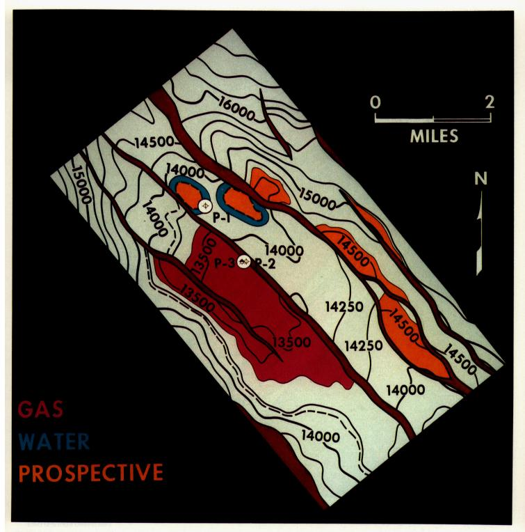
Fig. 8-3-2. Map of Pelican-3 sand interpreted from 3-D data with southeastern structural closure but not honoring water level in well. Contour interval 250 ft (76 m).
