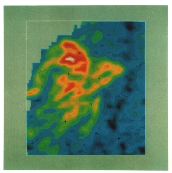
Fig. 2-22. Same horizon Seiscrop section as in Figure 2-21 displayed in a wider range of hues to draw attention to the high amplitudes using advancing colors. (Courtesy Chevron U.S.A. Inc.)
