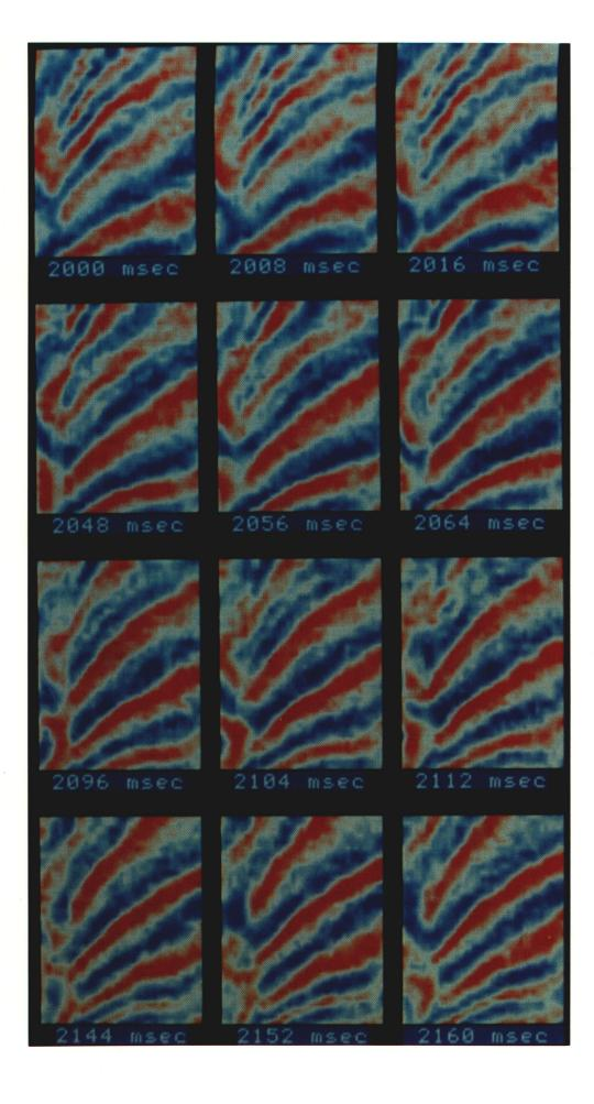
**Fig. 3-7.** The width of an event on a Seiscrop section decreases with increased dip and also with increased frequency.
