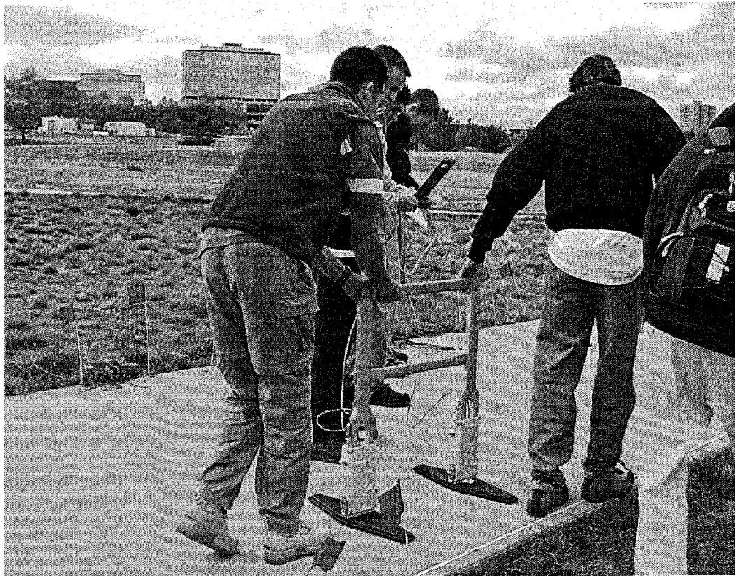
FIGURE 8.13 (a) Ground-penetrating radar profile showing inclined gravel. Time converted to depth using velocity of 0.14 m/ns. (Smith and Jol, 1992.) (b) GPR field equipment in use: Ramac system with 200 MHz antenna.
