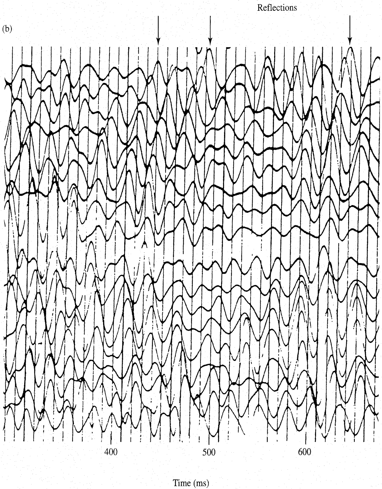
FIGURE 4.52 (continued) (b) Enlarged view of (a) to aid in picking reflection times.
