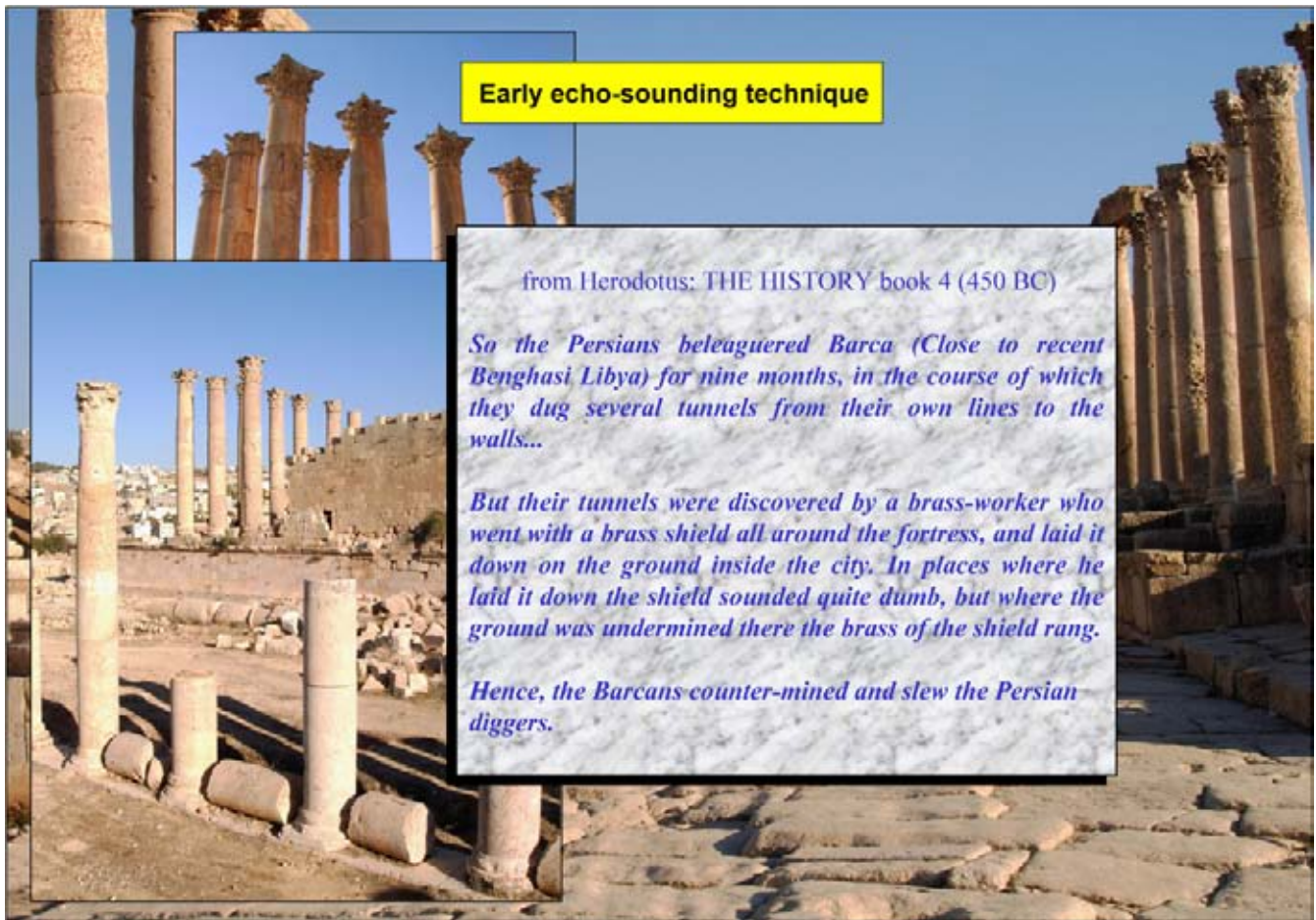
Figure 1.2: Extract from the book ‘Histories’ written by Herodotus of Halicarnassus around 450 BC, illustrating an early application of the principles behind the acoustic echo-sounding investigation technique (modified after Lawyer 2004).
