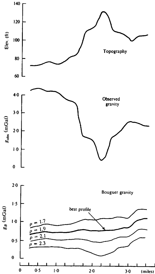
Figure 2.8. Method for estimating surface density.
